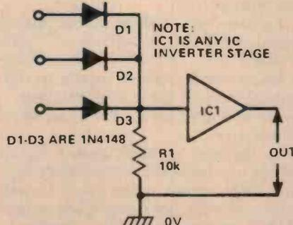
The diode OR gate can be converted to a NOR type by either feeding its output through an NPN transistor inverting stage, as shown in Figure 2a, or by feeding its output through any type of IC inverting stage that happens to be 'spare' in the circuit you are playing with, as shown in Figure 2b.
