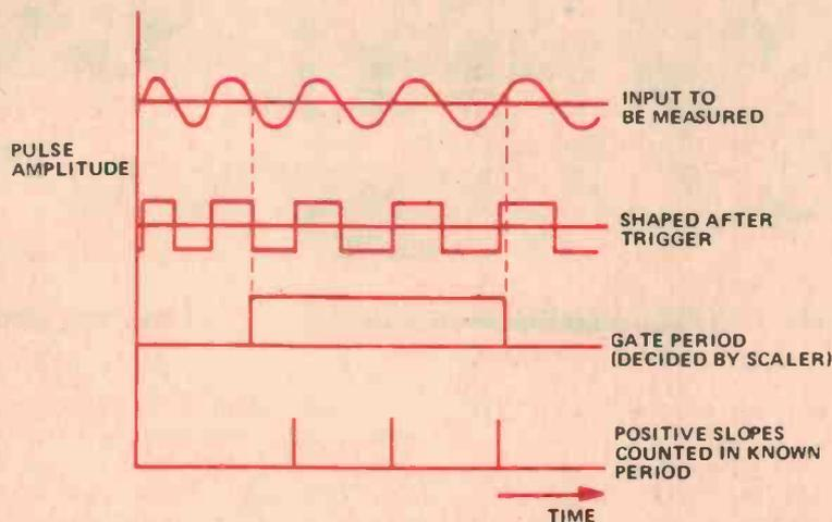
determined by the output from a divider/scaler driven by a very stable, accurate clock oscillator. A number of outputs from the divider/scaler may be selected to vary the period the gate is open. Usually, a number of decade steps are provided.
