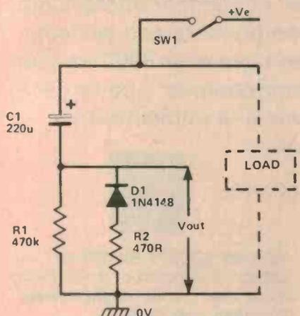
Figure 14. A basic variant of the Figure 12 circuit.
