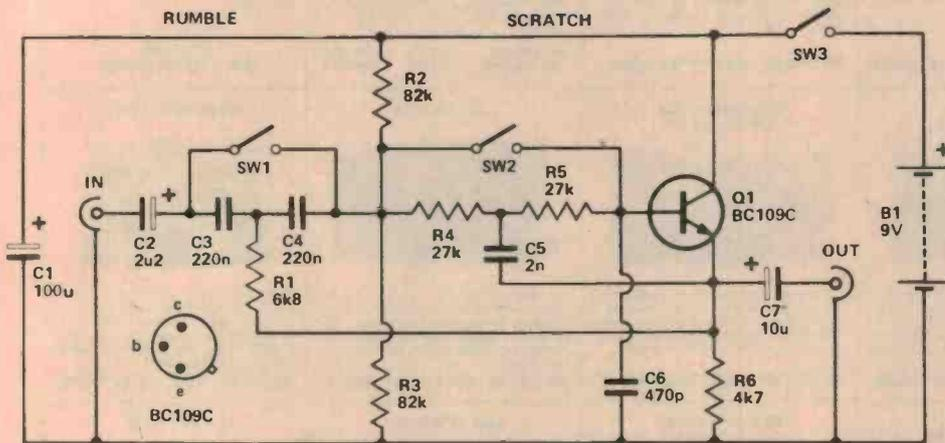
Circuit of the Scratch and Rumble filter. This unit may be mounted on matrix board and mounted inside your amplifier — don't forget two will be needed for stereo. If you construct it as an out-board unit it should be mounted in a metal box and connected into your amplifier system with short lengths of shielded cable. It may be connected between the "preamp out" and "main in" sockets.
