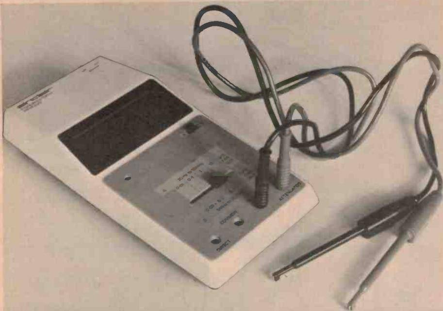
This handheld DFM from Sinclair Electronics features an eight digit display, two ranges — 20 Hz to 10 MHz and 5 MHz to 200 MHz, four gate times on the lower range and three on the top range. It is powered by a single No. 216 9 V battery and comes complete with input leads. Sinclair Instruments are available through Emona Enterprises, Suit 208, 661 George St, Sydney; Phone (02)212-4815.
