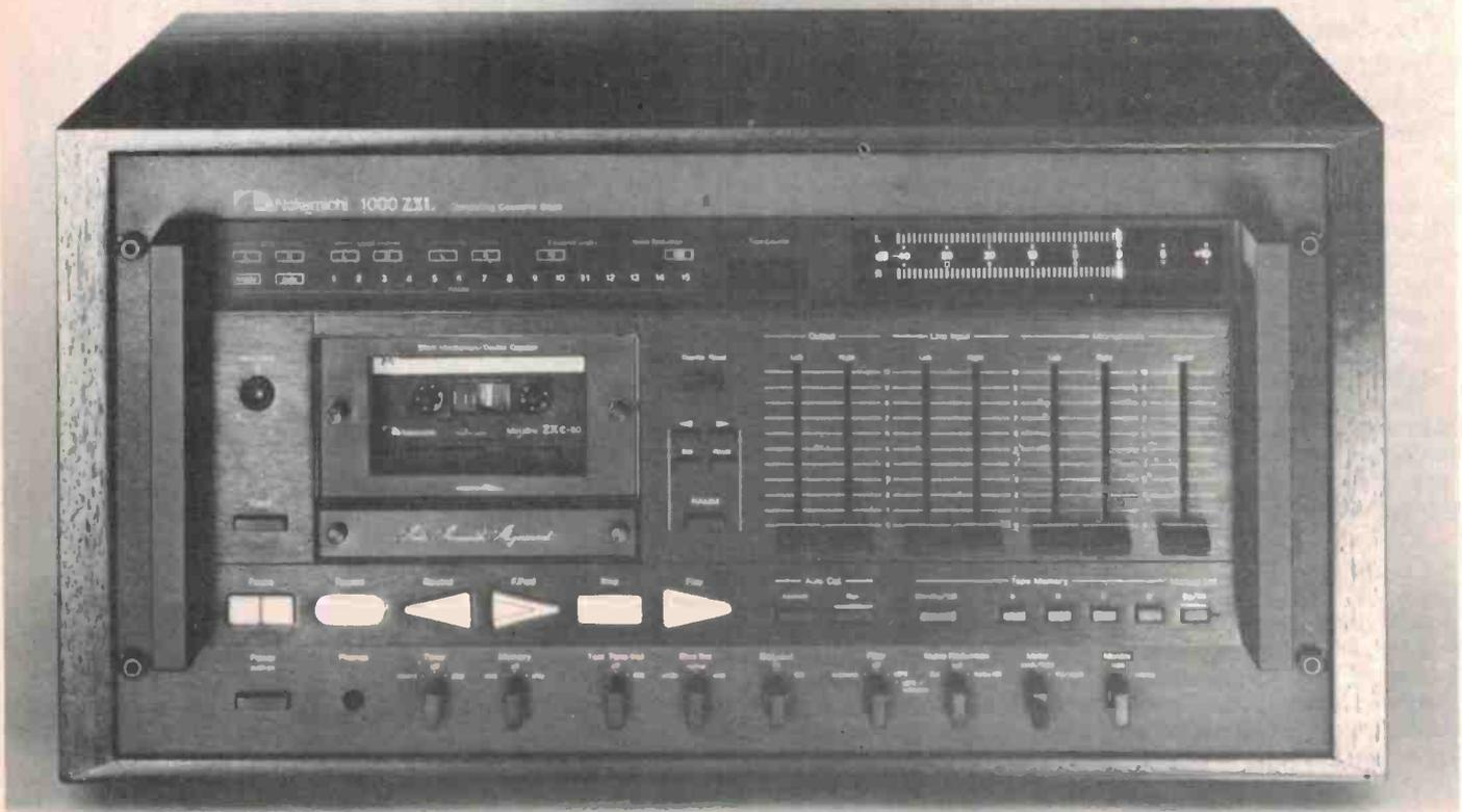
**The 1000ZXL has a microprocessor which independently controls tape head azimuth, bias, recording level and equalisation to optimise these parameters for the particular tape actually running in the machine.**
