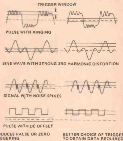
RIGHT: Trigger Setting Diagram. It is important to set the level of the trigger window such that extraneous signals on the main signal do not adversely affect the accuracy of the reading. Again, it is a good idea in many circumstances to examine the waveform with a CRO prior to making a measurement.
