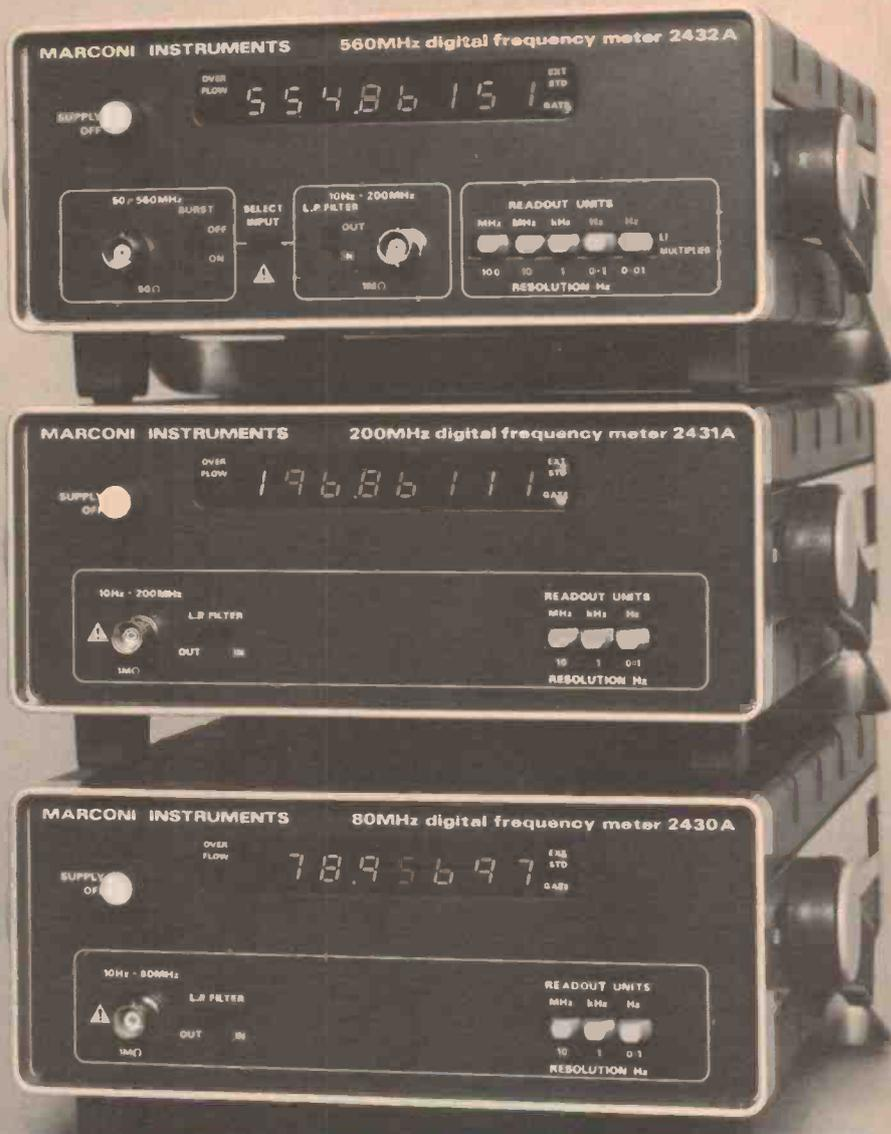
These three counters were recently added to the range of instruments offered by AWA. Made by Marconi Instruments, each features an eight digit display and a switchable low-pass filter. First in the range is the low cost model 2430A. It covers 10 Hz to 80 MHz and has three selectable gate times. The model 2431A (middle) covers 10 Hz to 200 MHz while the top-line 2432A includes a prescaler that permits measurements to 560 MHz, plus five selectable gate times.
