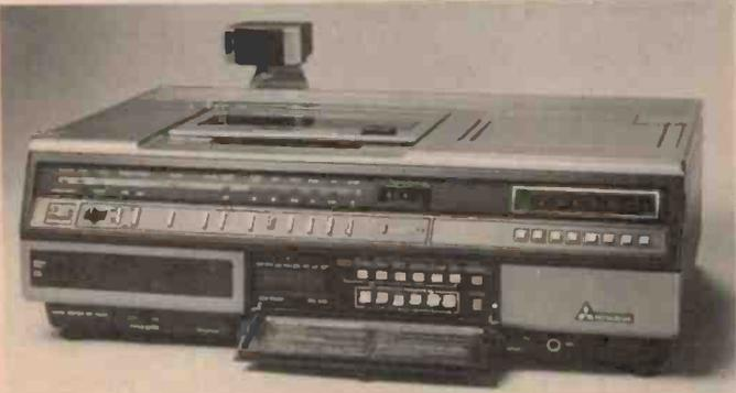
Facilities available on the HS 300 include fast picture search at seven times normal speed, slow motion search at half speed, freeze-frame, single frame advance and automatic rewind. In the freeze-frame and single frame advance modes the machine automatically searches for the most stable adjacent frame so as to avoid the picture deterioration often found in other VCRs operating in these modes.
