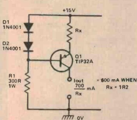
Figure 11. A simple and very useful current generator.
