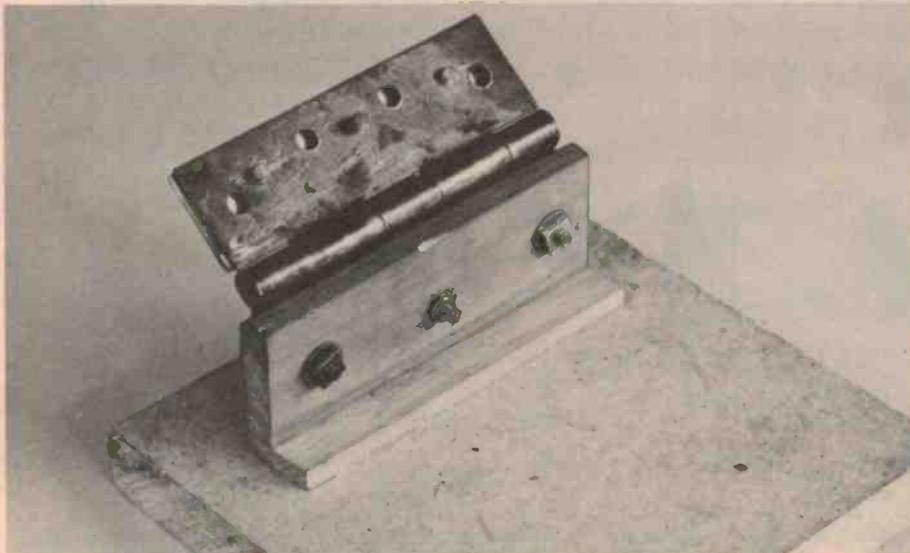
The accompanying photos show the "spare hand" in the up i.e. 'load components' position, and — minus the circuit board, in the down, or 'solder' position.
